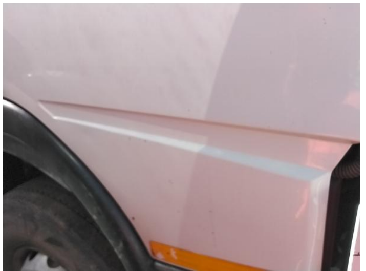
12: Door osf Chipped Multiple Chips
